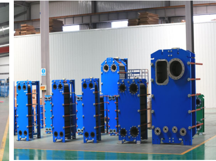
Finished Plate Heat Exchanger
