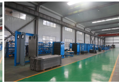
Plate Heat Exchanger Workshop
